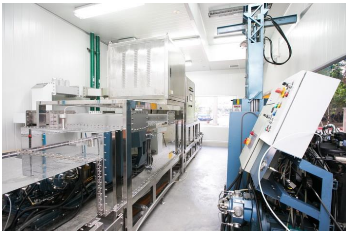
Radio frequency fish thawing machine
